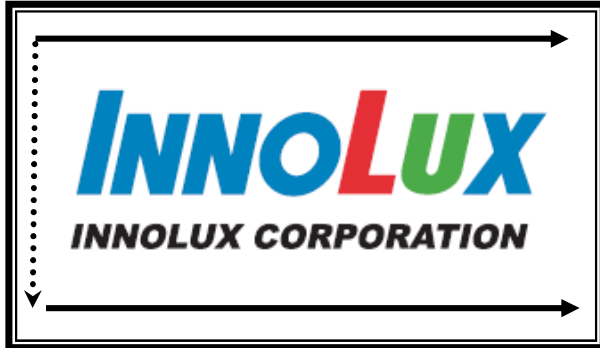
Fig. 1 Normal scan ( pin 4, LR/UD = High or NC )
